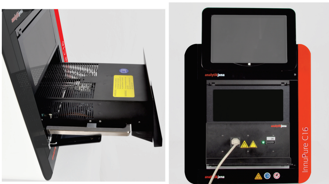
Fig. 6 Inserting lamp into InnuPure C16 touch , connecting and switch-on
