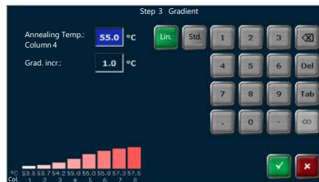
Twin block: The gradient is vertical. "Column" (line) 1 starts at the bottom left.
